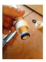
C. Feed the pipe into the opening where the piezo is based, and gently with a screwdriver you can squeeze the 'o' ring into the opening.
